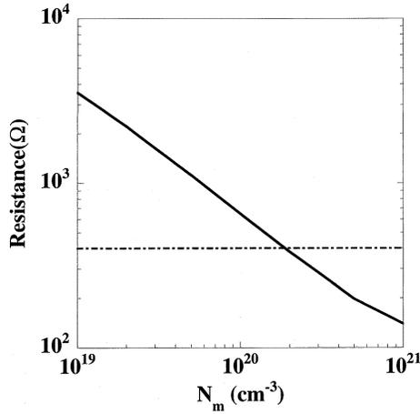
Fig. 7. Dependence of sheet resistance on  $N_m$ .
