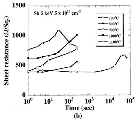
Fig. 2. Time evolution of sheet resistance. (a) 450, 500, and 600  $^{\circ}\text{C}$ . (b) 700, 800, 900, 1000, and 1100  $^{\circ}\text{C}$ .
