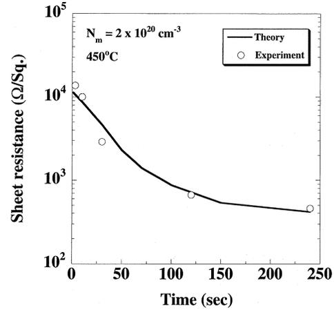
Fig. 9. Comparison of experimental sheet resistance on time with our model.
