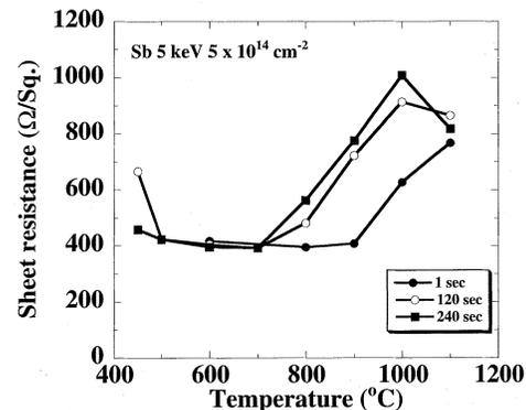
Fig. 1. Dependence of sheet resistance on temperature.
