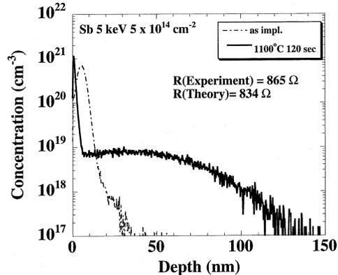
Fig. 11. Concentration profiles for Sb diffusion at 1100 °C.
