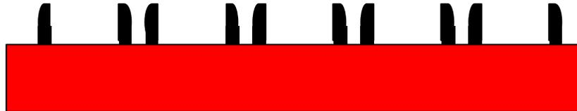
(d) Selective etching away the dummy material. Oxide spacers are left. Adjusting the dummy material thickness controls the oxide hard mask height.
