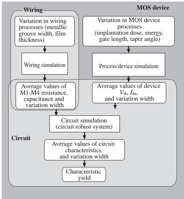
Fig. 4—Raising Robustness of Circuits and Devices at Development Stage.
