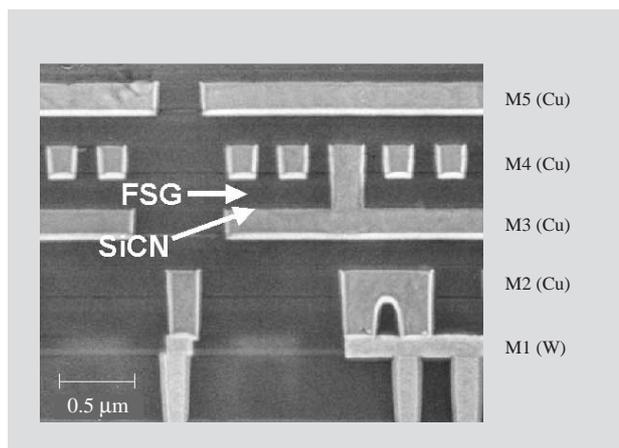
Fig. 3 —Cross Section of 0.36- $\mu\text{m}$ -pitch Cu Wiring. Hitachi uses Cu wiring with a 0.36- $\mu\text{m}$  pitch for a 130-nm-node CMOS, as well as fluorine-doped silicon oxide as an inter-layer film and SiCN as a Cu-barrier film to reduce permittivity.
