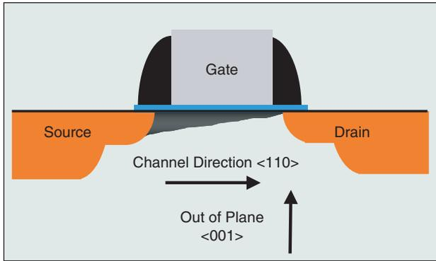
1. MOSFET schematic device cross section (standard orientation).
