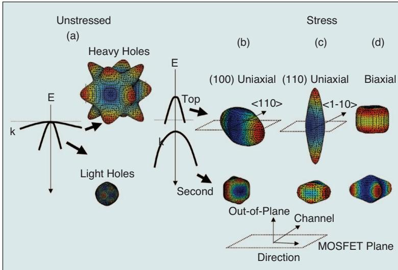
3. Hole constant energy surfaces at 25meV obtained from six band  $kp$  calculations for common types of stresses: (a) unstressed, (b) longitudinal compression on (100) wafer, (c) longitudinal compression on (110) wafer, and (d) biaxial tension.
