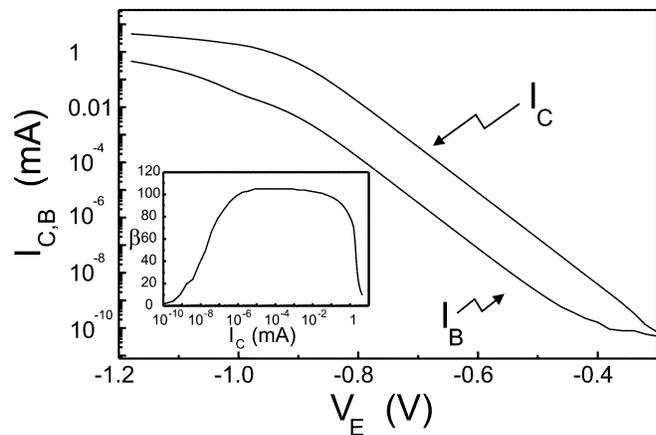
Fig. 8. Typical Gummel plot with corresponding current gain (inset) for a  $0.22 \times 1.20 \mu\text{m}$  transistor of type A.
