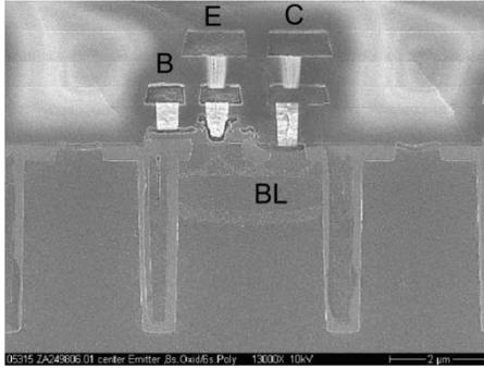
Fig. 4. Cross-sectional SEM micrograph of the self-aligned SiGe base bipolar transistor in a base(B)-emitter(E)-collector(C) arrangement. The buried layer is decorated to become visible.
