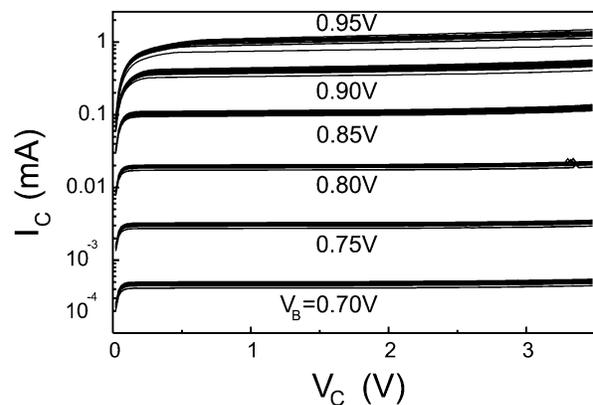
Fig. 9. Output characteristics for 16 HBTs of type A (effective emitter area  $0.22 \times 1.20 \mu\text{m}$ ) at different base-emitter voltages  $V_{\text{BE}}$ . At low collector currents an early voltage around  $-200 \text{ V}$  can be deduced.
