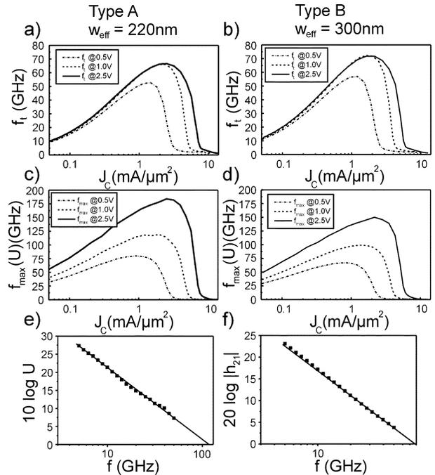
Fig. 6. (a), (b)  $f_t$  and (c), (d)  $f_{\text{max}}(U)$  for the type A and B transistor ( $A_{\text{eff}} = 0.22/0.30 \times 7.6 \mu\text{m}^2$ ) at different collector-emitter voltages. (e), (f) shows the extrapolation of  $f_{t,\text{max}}$  and  $f_{\text{max,max}}(U)$  at  $V_C = 1$  V for type A and B, respectively.
