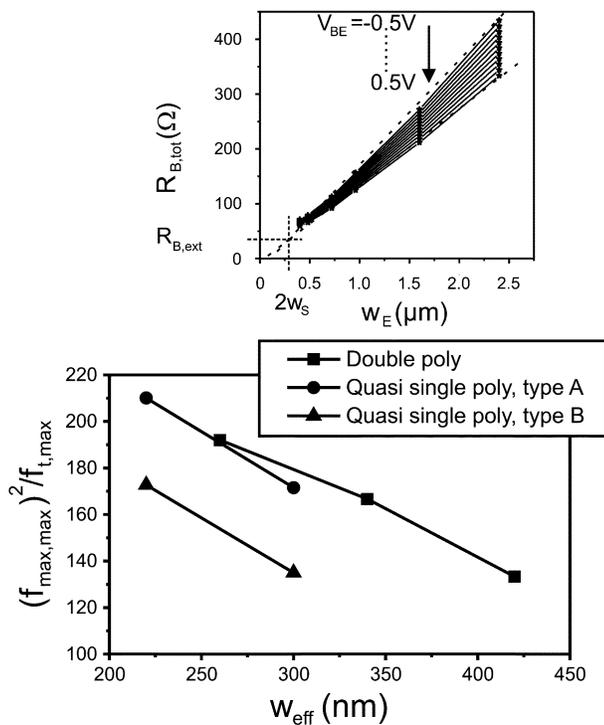
Fig. 7.  $f_{\max,\max}(U)^2/f_{t,\max}$  versus effective emitter window width  $w_{\text{eff}}$  for both types of quasi-single-poly HBTs and also conventional double-poly HBTs for comparison. The upper inset shows  $R_{B,\text{tot}}$  of a type A HBT as a function of  $V_{\text{BE}}$  for different  $w_E$ . These traces serve to derive  $R_{B,\text{ext}}$  as described in [18].
