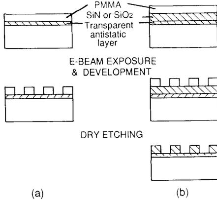
FIG.2. Process sequence of transparent phase shifting mask with (a) polymeric shifter (PMMA) and (b) inorganic shifter (SiN or SiO<sub>2</sub>).
