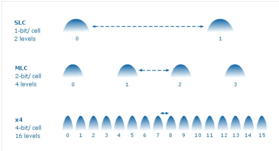
*Figure 3: Voltage Levels in 1-Bit, 2-Bit and 4-Bit/Cell Technologies*
